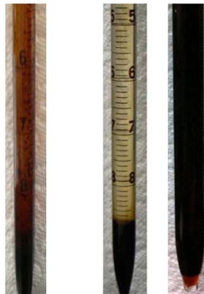
Postmixing Non-catalytic oak oil mixing with tetralin Premixing 4g 5% Ru/TiO 2 catalyzed oak oil mixing with tetralin Postmixing 4g 5% Ru/TiO 2 catalyzed oak oil mixing with tetralin
