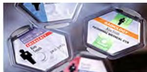
A radiation dosimeter that is now used in hospitals and nuclear facilities worldwide is the result of EPSCoR-initiated research. Last year more than 1.8 million workers were protected from radiation exposure by the monitoring device. The product generated over \$104 million in revenue during fiscal year 2016.
