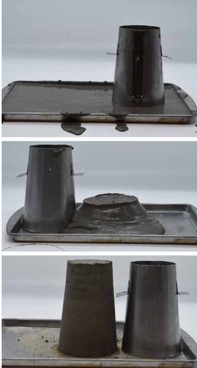
Figure 1. An example of slump testing of tailings at (a) 65 percent, (b) 75 percent, and (c) 85 percent solids contents (solids content = weight of solids/total weight). (Photo courtesy of Kendall Monley.)
