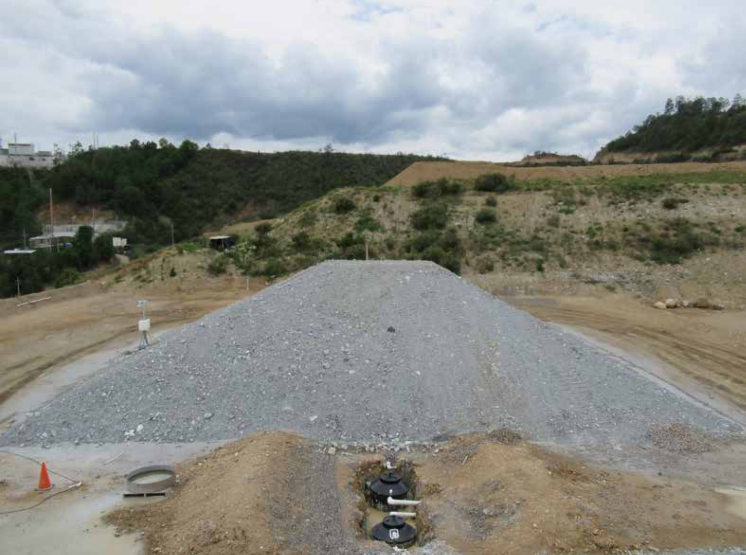
Figure 4. Commingled filtered tailings and waste rock test pile.
